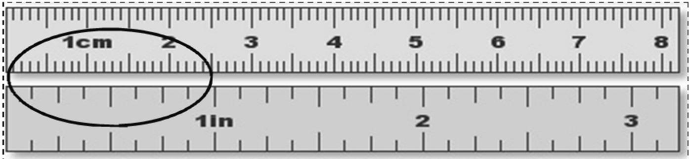
In this close up of two rulers, top metric (mm and cm), the bottom in English (eighths of inches & inches). If we try to measure the length of the oval, we could say it's about 1 inch long. Or we could measure it to be 2.5 cm, or 25.0 mm. The smaller the increment, the more accurate the measurement.
