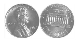
Objective: To discover the unknown metal inside of the new pennies, which changed from being ALL COPPER before 1982, to just 2% copper plated over this "unknown" metal inside since 1983. You will measure the old pennies to sharpen your skills, and then carefully measure the new ones to try and discover what this unknown metal is.
