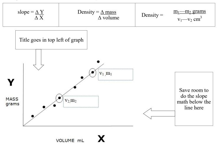
Circle and label  $(v_1, m_1)$  as well as  $(v_2, m_2)$  on BOTH of your graph lines. These are the points you are using in your slope calculation. Only use points that are ON THE LINE.
